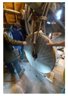
3 inches between the ends of the beams and the upright runner stone. The beams should be about 2ft apart and placed with the narrow side down, as shown below. The important point being that the upper edges of the ends of the beams are well within the face of the stone. See the sketch below. This is so that when the stone is lowered, the weight of the stone bears on the front ends of the beams and not the inside edges.
