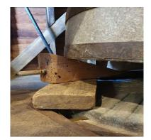
As the runner stone is lowered, it is also important to make sure that the slots in the mace remain aligned with the rhind.
