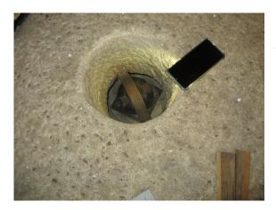
The picture shows the runner stone centred over the bed stone. At this point the mace must be rotated by hand so that the curved indents in the mace are aligned with the rhind. The rollers can now be removed so that the runner stone is sitting on the long beams.
